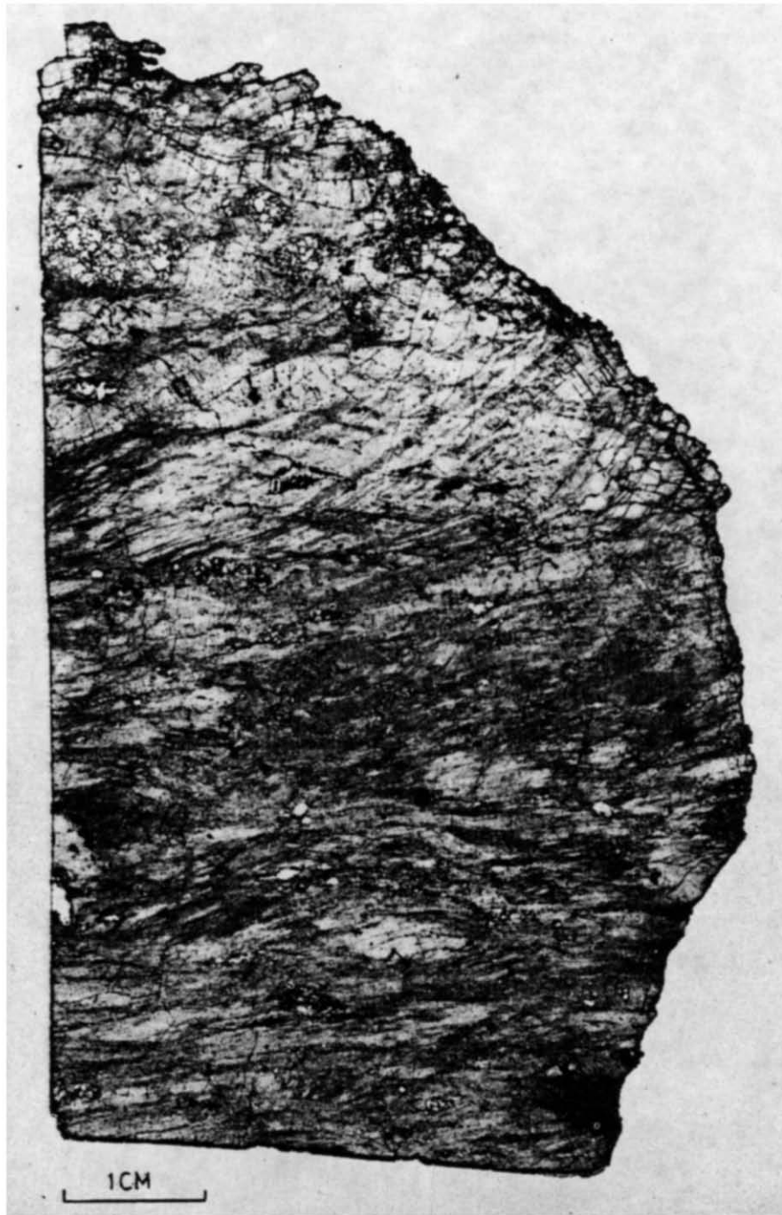
Fig. 1. Photograph of an acetate peel of a sample of sheared galena from Yerranderie, NSW. The sense of shear is dextral. Note the curving foliation delineated by kink bands. Section cut normal to the foliation and parallel to the lineation (horizontal).
